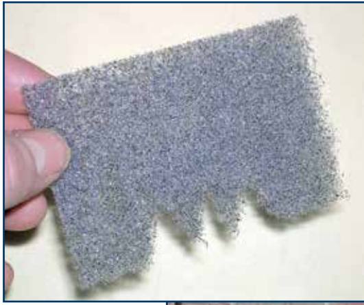
Figure 9 – Polymer mesh weep vents located 8 in. on-center for more drainage and drying capacity for this veneer replacement. The original unventilated veneer showed signs of distress after only eight years. Much of the water source in the wall cavity came from condensation of uncontrolled moist interior air from this densely occupied office building in a northern climate.
